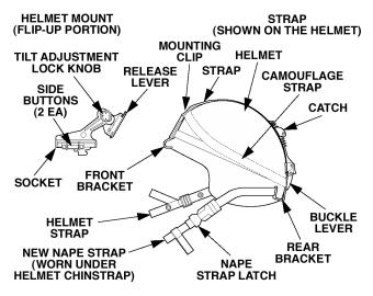
Figure 2-20. Helmet Mount Features (New Nape Strap).
